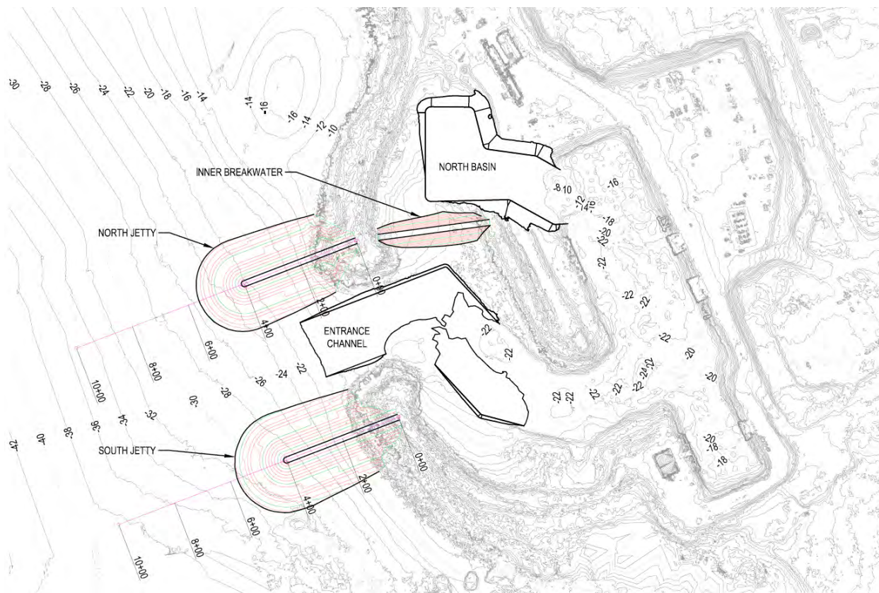
Example of an alternate harbor geometry tested by USACE's nested model
